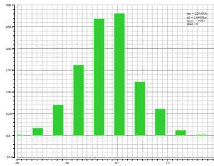
Figure 5: INL distribution for a 1000 run monte carlo test
