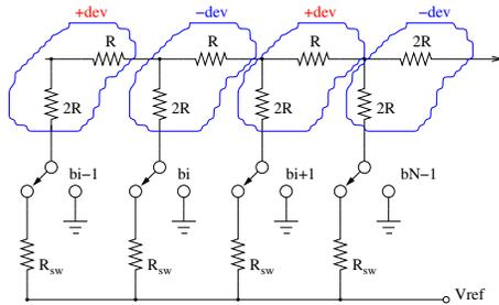
Figure 3: INL due to mismatch in adjacent sub-stages
