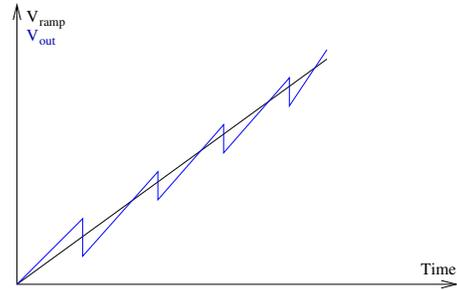
Figure 4: INL deviation due to mismatch in adjacent sub-stages
