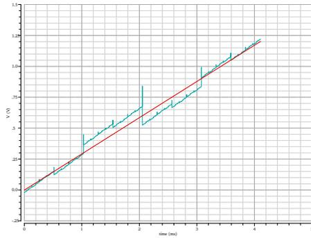
Figure 6: Mismatched DAC's ramp transfer function
