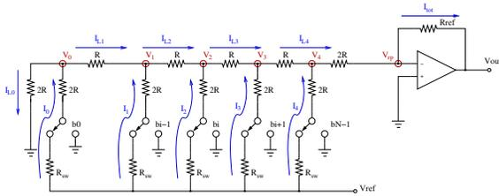
Figure 1: Current distribution in an R-2R DAC
