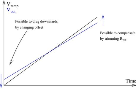
Figure 2: INL in the abovementioned 2R-2R mismatch case and a way of compensating the errors from this case
